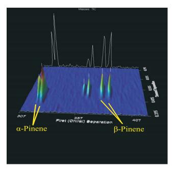
Figure 13. GCxGC surface plot of early eluting enantiomeric pairs showing good separation in the first chromatographic dimension.
