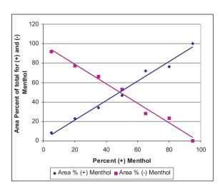
Figure 12. Response (area %) for menthol isomers as a function of weight percent of (+)-menthol, as determined using GCxGC.
