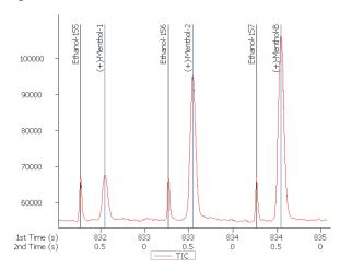
Figure 9. A portion of the GCxGC linear chromatogram through a (+)menthol peak represents successive second dimension chromatograms of the eluent from the first dimension column.
