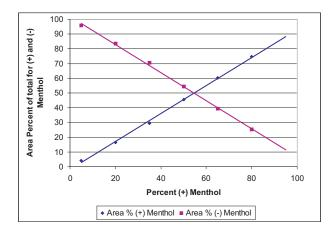
Figure 8. Response (area %) for menthol isomers as a function of weight percent for (+)-menthol, as determined by one-dimensional gas chromatography.
